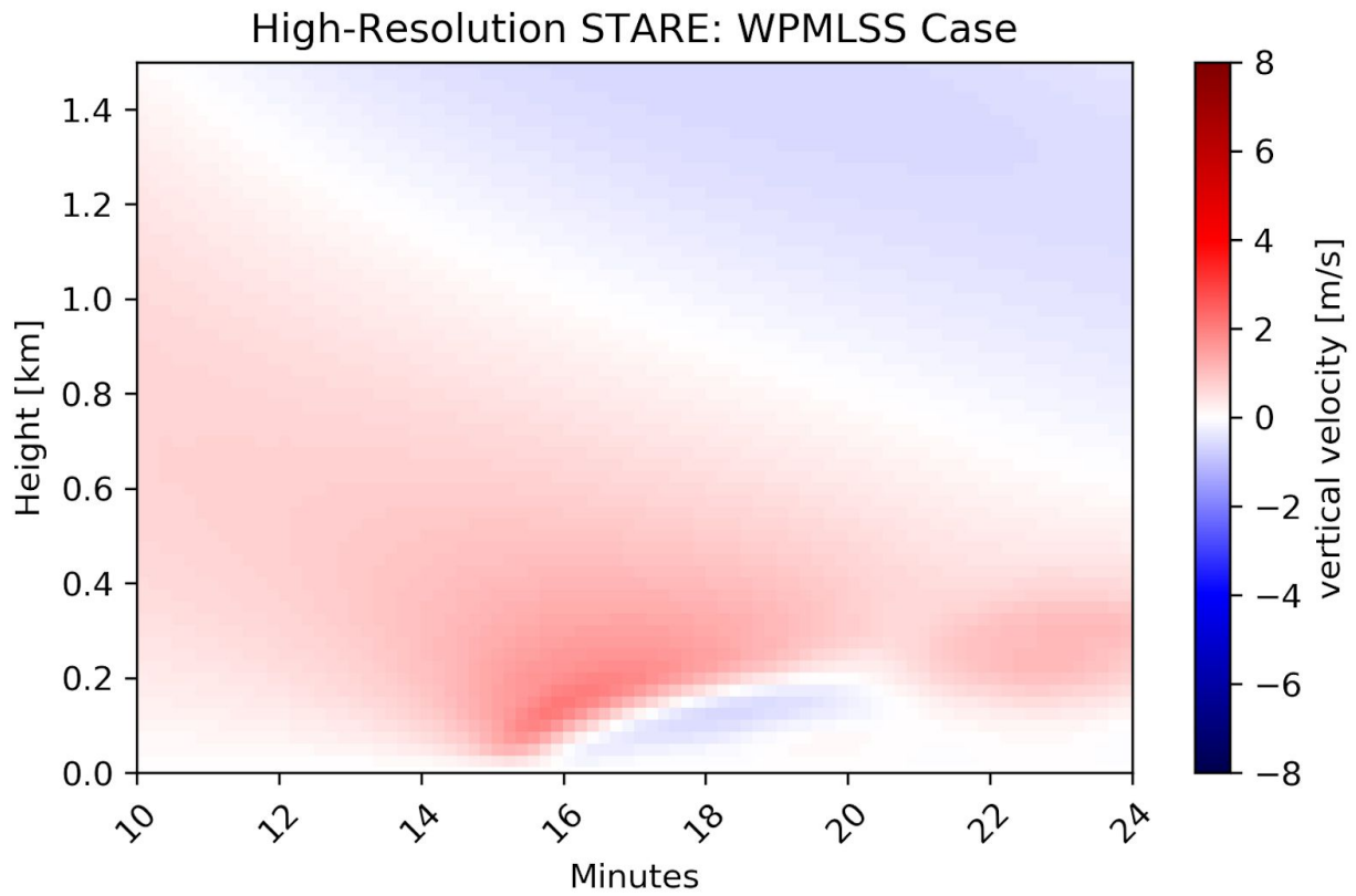
Figure 7: Simulated high-resolution stare from the weak perturbation - medium potential temperature lapse rate - strong shear simulation. These environmental conditions closely represent those observed from the TORUS field campaign on May 27, 2019 in Imperial, Nebraska.
